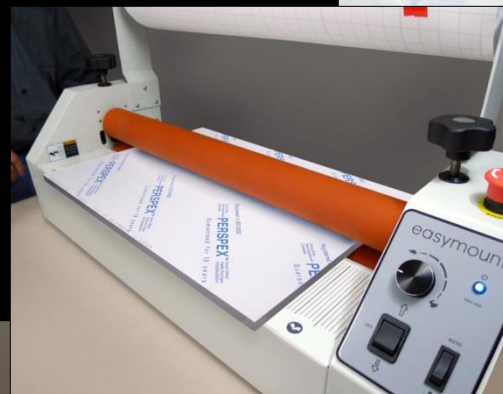
3. Place the acrylic under the print and verify alignment of all layers. In a single motion, feed through RL peeling the release film.
