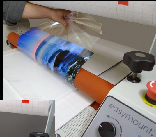
4. Pass acrylic through RL to fully adhere edges.
