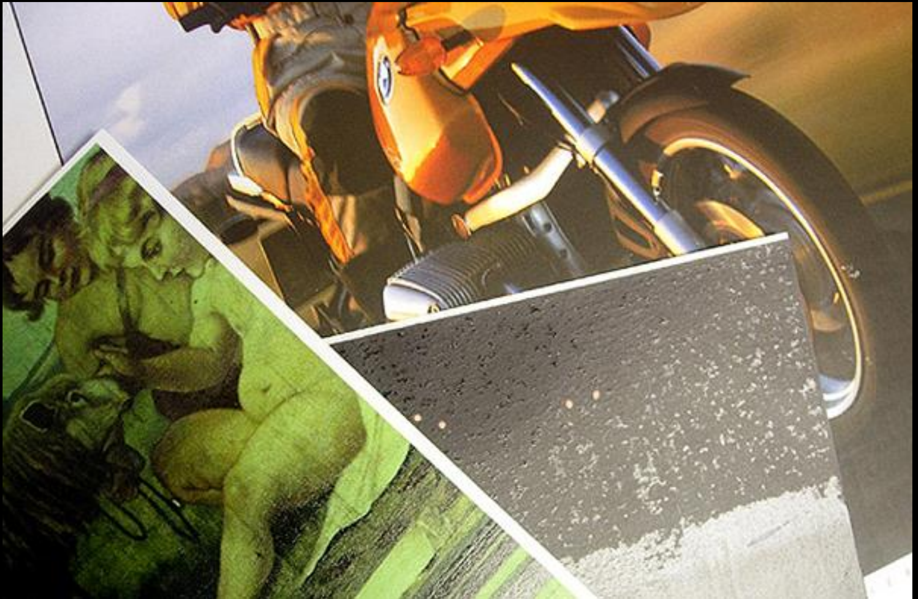
Electrophotographic four color toner copies and heat damage
