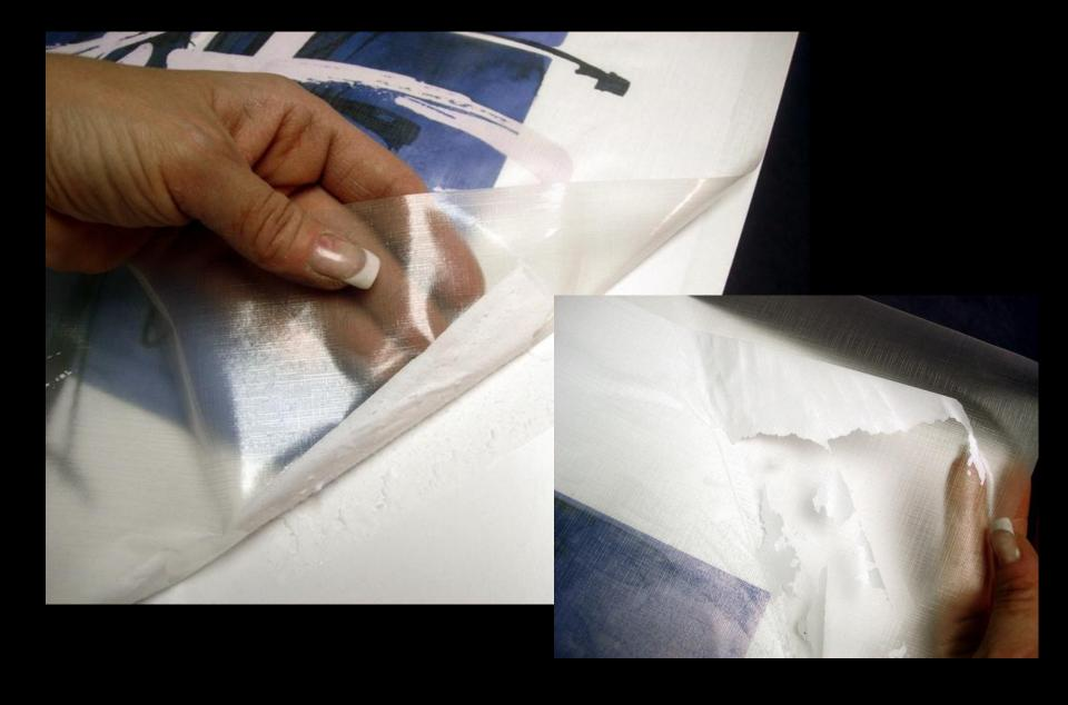
Digital press toner lifts ink from paper when laminate is lifted to realign
