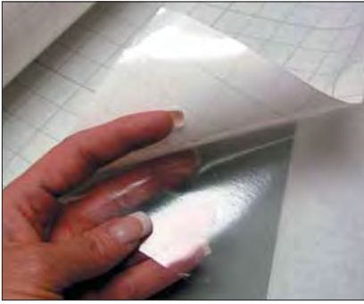
Photo 2: All vinyl laminating films have a layer of lightly tacky heat activated adhesive applied to the back side with a single release liner. Save the liner when removed for retexturing of the surface.
