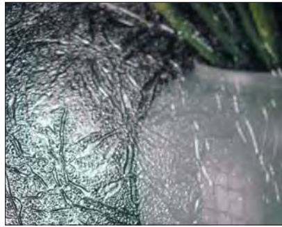
Photo 15: Regular clay coat foamboard and glass laminate will produce a wrinkle that depresses into the board giving a deeper wrinkled effect, and the glass shows more texture.
