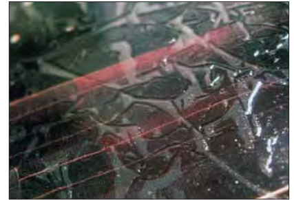
Photo 7: When overlay foam has been forgotten from the laminating package trapped air pockets will result.
