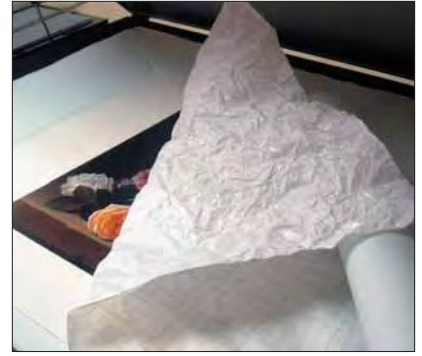
Photo 13: Place the wrinkled liner over the mounted/laminated print, without sponge foam and run through a full press cycle.
