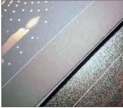
Photo 9: The left upper half of the photo shows a print with ultra matte laminate that does not exhibit sponge texture, while the lower right half glass does showcase the texture.
