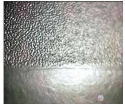
Photo 10: The act of removing the embedded sponge texture from a laminate surface is called resurfacing. The upper half of this print shows the typical sponge texture while the lower half has had the texture removed by remounting with the laminate liner laid over the surface.
