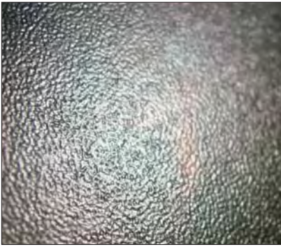
Photo 8: When correctly mounted, the soft vinyl laminate will pick up the open cell texture of the overlay foam during the mounting process.
