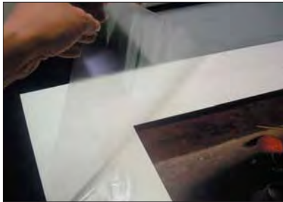
Photo 5: Lift the film from each end, and roll back down onto the print to generally smooth out air.
