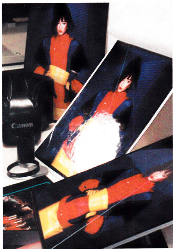
Photo 1: Ilfochromes will show orange peel regardless of wet, spray, pressure-sensitive, or dry mounting as seen in the light reflection on the middle photo. The left half was dry mounted; the right half was spray mounted.
