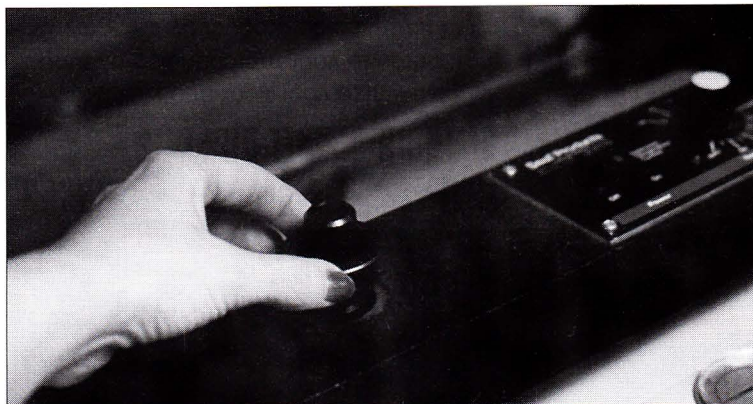
For permanent readjustment of a mechanical press, loosen the outer locking ring and turn the tall inner adjustment knob to loosen or tighten press pressure — or use shims instead.
