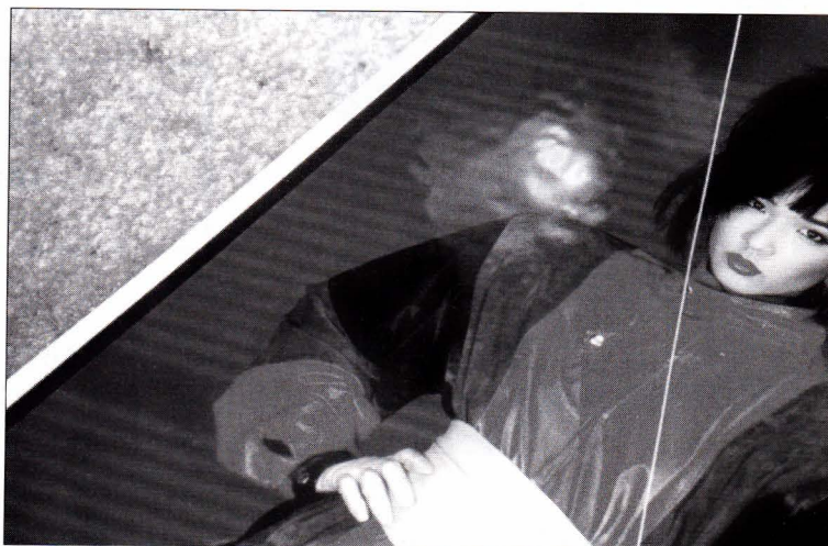
Orange peel, though difficult to photograph, is seen on the left half of this mounted cibachrome where the light is reflecting. The photo has relaxed to match the contour of the substrate.
