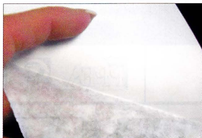
Photo 4: Once split, the paper core may be peeled back separating the image from the support materials much as with any traditional RC photo, exposing the sheer nature of the thin-coated backing.
