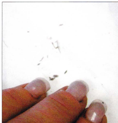
Photo 7: Normal maintenance and cleaning of release materials is easy. Once adhesive has cooled, it may be brushed off with a clean lint-free rag or with your fingers, as shown in this photo.
