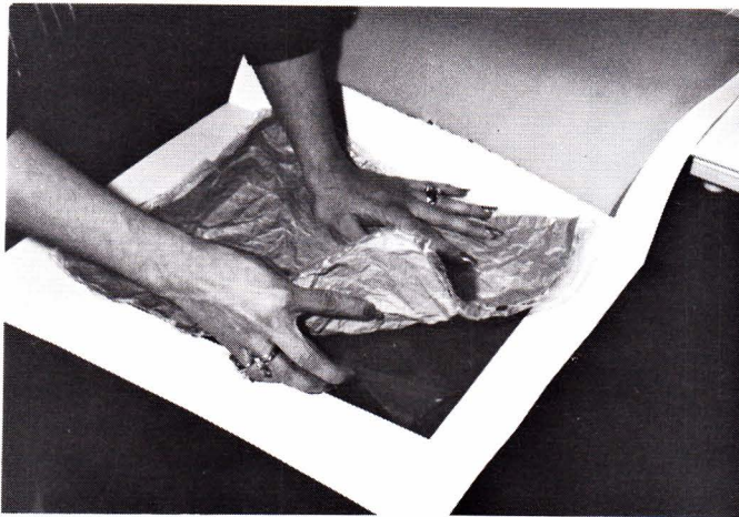
7. Place a sandwich of overlay foam, wrinkled and flattened laminate/art paper, pure adhesive, and mat board in an envelope of release paper and place into a mechanical or hot vacuum press for 5 minutes (adhesive and board should be 1" smaller than the laminate).
