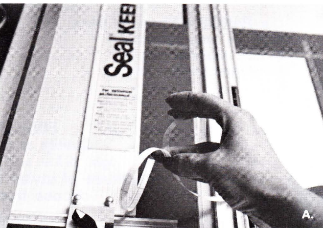
4A., B. Peel backing paper from the laminate and lightly tack the strips into place on the face of the mat along the cutter bar. Let the strips extend to just short of the full length of the mat so adequate laminate is available for mitering.
