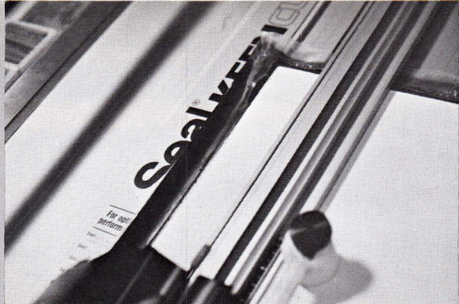
Photo 4. Cut the foam board face down, end for end, for all four directions. Make certain not to cut through the face layer of the foam board or the fabric, since these will serve as hinges for the sides of the box.
