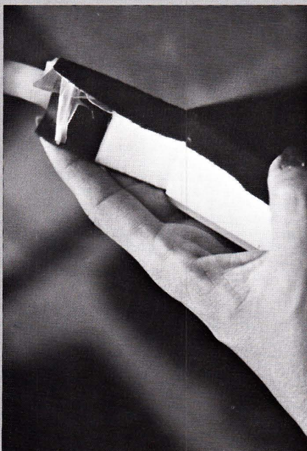
Photo 9c. By tacking the turnback first, the tab turns cleanly and is ready to be taped.
