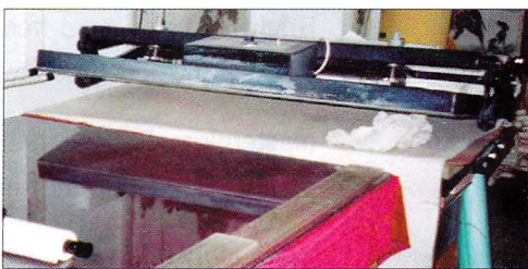
Photo 5: This is a Chinese manufactured 48" wide (equivalent) mechanical press very much like the Bienfang presses in the U.S. They have a felt sheet covering the bottom, and there is a rag that is used to wipe down the press between mountings. It has a sponge pad layer like those used here.
