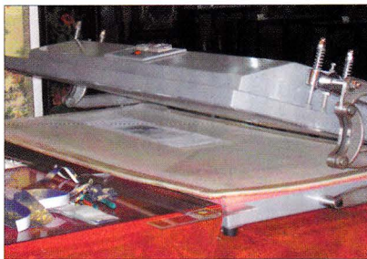
Photo 8: This clean press is well taken care of. The bottom of the press has a release paper covered, homemade, wrapped pad to protect the sponge beneath it. Note the cut brocade strips the left of the press ready for mounting.
