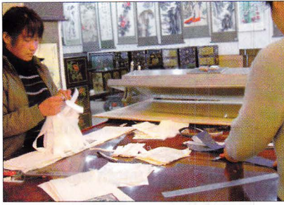
Photo 6: Just as U.S. framers tack images to the backing board of choice, these production framers attached brocade strips to the color accent trimmed original painted image, which will then be placed in the press for final fusion.
