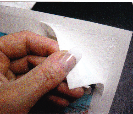
The mounted polyester encapsulated map tears the top layer of adhesive and paper from the board after mounting, illustrating perfect tear strength
