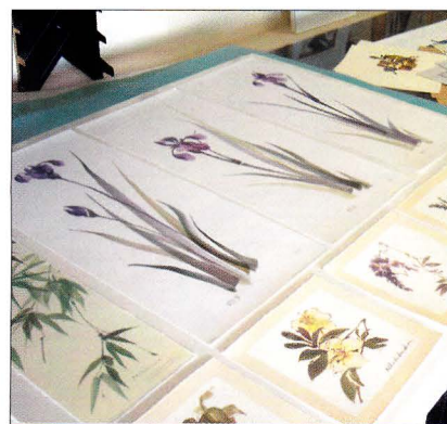
Photo 4: A full sheet of heat-activated Step 150 foamboard is fitted with as many assorted prints as possible to make each press run as economical as possible.
