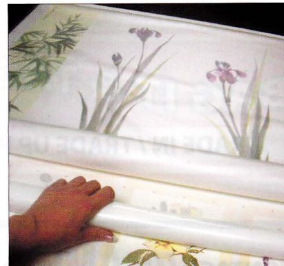
Photo 7: This sample was mounted first to prevent image shifting, then one full sheet of laminate was applied over the entire board for an additional press run. The top end is aligned while the liner is being peeled off from under the stuck film, which is hand rolled for easier handling.
