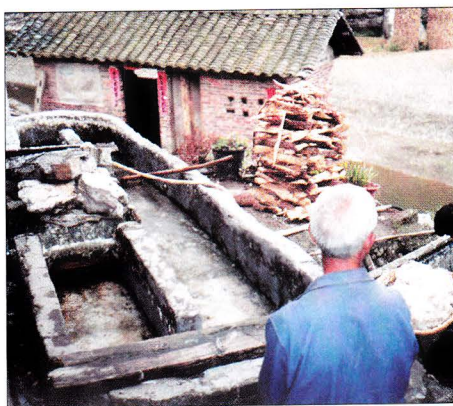
Photo 5: The antiquated looking grinder is made entirely of stone. Softened fibers are placed upper left into the hand grinder that pulverizes and breaks down the fibers into pulp mash. The mash runs around the top end of the downhill trough to the lower right corner where excess water runs into the river and the pulp is harvested for carrying to the vats.
