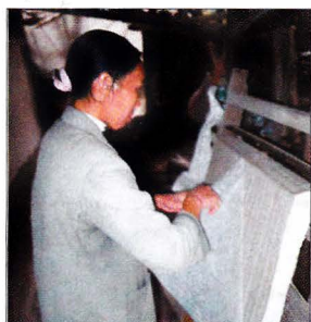
Photo 11: Pressed sheets are removed one by one from the pile by gently peeling them apart while lightly moist. Papers vary in thickness as in one, two and three ply thus catering to the needs of the user. Photo 12: Separated sheets are adhered to a smooth, heated stone wall to dry and using a stiff 12" wide palm bristle brush to remove all air beneath. Sheets may be one-, two-, or three-ply thick depending upon the request of the buyer
