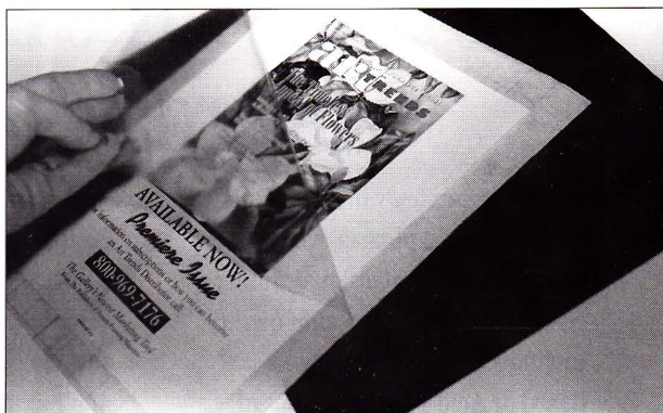
PHOTO 6 Trap the magazine page between the liner and perforated film, using the gridded liner as a backing.
