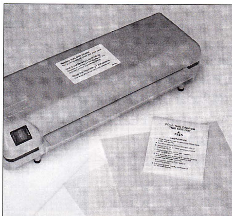
Photo 4 Commercial office laminators are manufactured by numerous different companies and are available in a variety of standard sizes. Polyester pockets of film are fed through a set of heat rollers inside a release material carrier as pictured.
