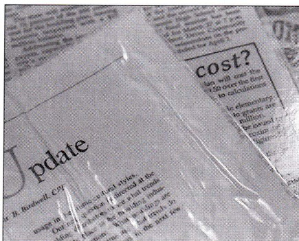
Photo 12 Curling after step one mounting can make alignment and mounting of side two very difficult.
