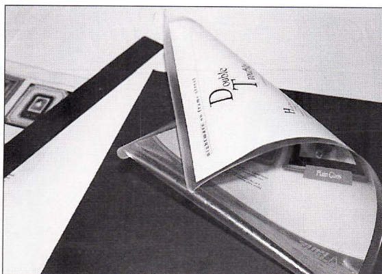
Photo 11 The front left sample was never cool beneath a weight and remains very stiffly buckled. This will never be flattened now, even with reheating. The center sample is the front side of an encapsulation of breathable newspaper, cooled under a weight. The detail at far right though cooled under a weight (as the breathable newspaper) is a non-breathable sheet and clearly illustrates trapped air even on side one.
