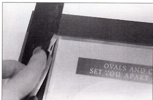
Photo 10 If attempting to encapsulate with polyester films, cut both sheets prior to mounting for exacting sizing and more control.
