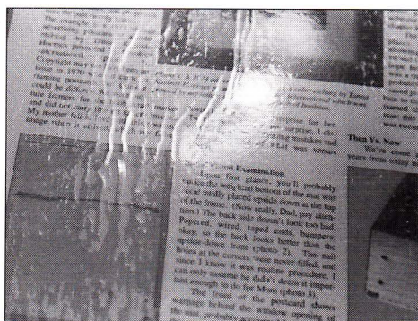
Photo 13 This is it. All the right things done, as directed...and still unacceptable. Clouded trapped tunnels of air and polyester rippling.
