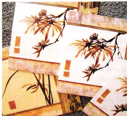
Photo 2: At the lower left is a yellowed laminated image. At the top center is the 185°F mounted image with a pale yellow halo. At the right is a 160°F mounted image without any yellowing.
