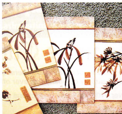
Photo 3: Comparing: Bienfang Finish Guard Linen (left); Drytac ArtShield Satin Matte (center); mounted at 160°F to Speedmount; and an unmounted, unmounted print (right).
