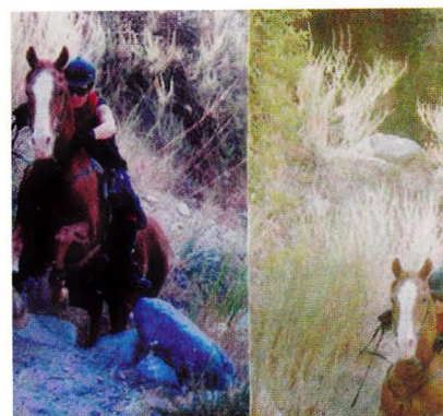
Photo 8: Inkjet fading is a reaction to UV and visible light that causes inks to fade, leaving the yellow dominant in digital prints. This damage seen here is not due to framing.
