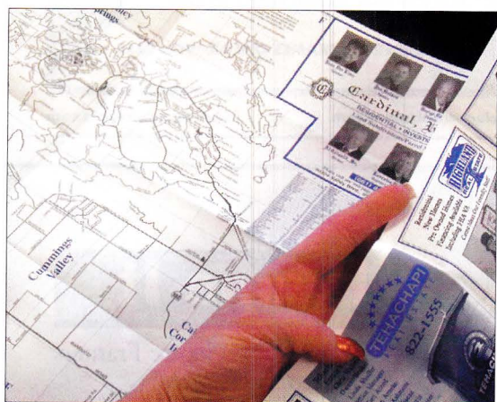
Photo 1: A 30"x18" real estate map is printed on two sides with heavy solid areas of blue and black ink on the back. It is new but has bold folds and heavy ridges because of the heavier weight paper.
