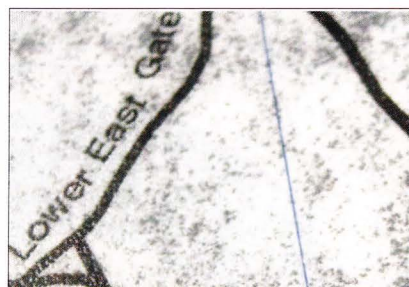
Photo 16: This laminated sample was left in the press for nearly 20 minutes while a customer was being helped. The adhesive saturation left blotchy spots across the surface of the map, which meant starting again.
