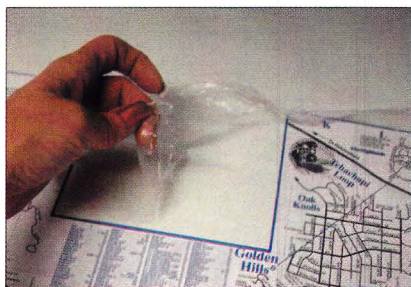
Photo 5: Drytac Flobond is self-shaping. When the top release paper is lifted from the mount, the trim adhesive may be easily lifted from the sheet and will break off to the edges of the odd-shaped map.
