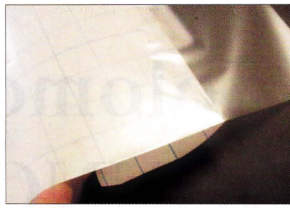
Photo 9: Fold back the top few inches of the release liner backing attached to the laminate to expose the tacky adhesive on the underside of the laminate.
