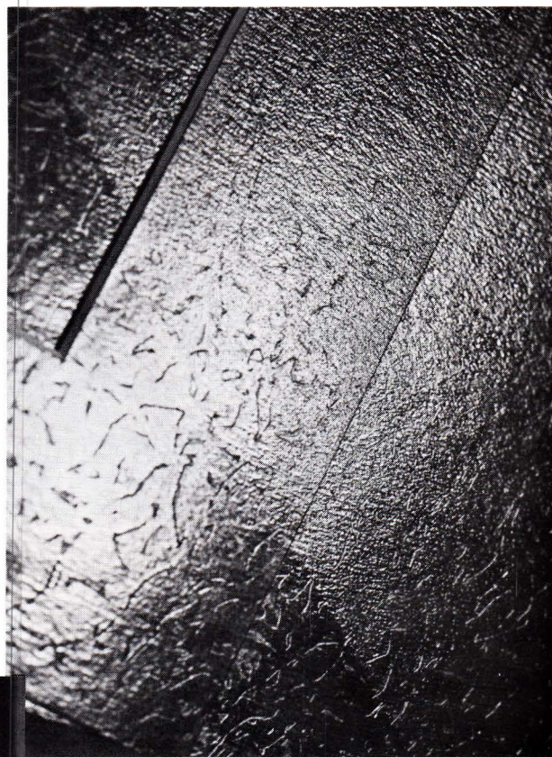
Photo 5. The mat (at a high glare photo angle) in photo 5 shows the extreme difference in double pressing first with foil/foam, second foam only. Notice the reduction of texture and increase in luster.
