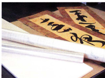
Photo 3: Materials—The basic materials selected for this project included \frac{1}{2} " foam board, rolled dry mount adhesive, and satin-matte finish surface laminate.
