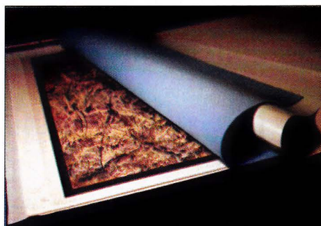
Photo 2: Overlay foam (a.k.a. foam plastic) must always be used when laminating. Many films will react with the silicone of the release materials as seen in the center.
