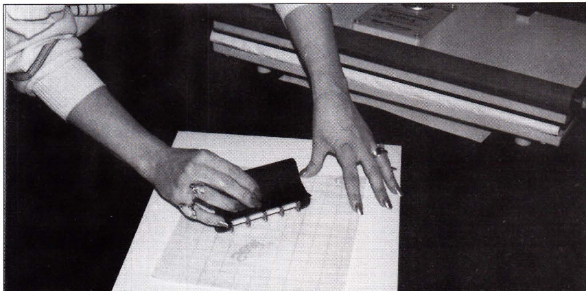
Photo 4 Manual perforation is executed with the film face up to prevent tufts of the paper backing from remaining stuck in the holes.
