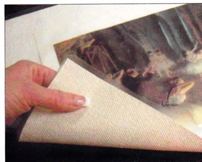
Photo 13: The new laminate decal/HA canvas unit may now be placed in the press for bonding.
