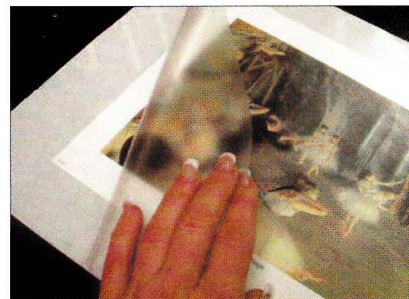
Photo 4: Roll the laminate back over the print and close it against the release liner.
