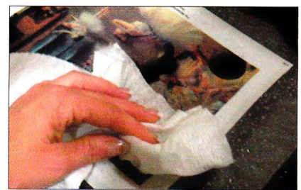
Photo 7: After 15 minutes, remove the print, shake off additional water and place it face up on a hard Formica or glass-top surface. Dry off the print and flatten it against a table, sopping up excess water.
