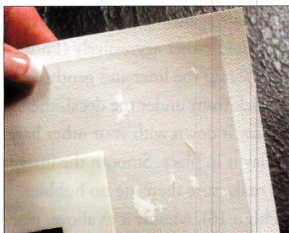
Photo 14: This exposed adhesive would bond to the sponge during mounting.
