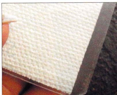
Photo 12: Make sure all of the HA canvas has been covered by the laminate so it does not adhere to the sponge.
