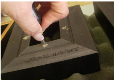
photo 12 - Countersink Preparation Use whatever method works for you. Use a larger phillips head driver to twist and enlarge the small pilot hole removing additional wood to accommodate the head of the screw.
