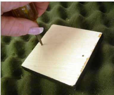
photo 16 - Starter Holes in Platform
