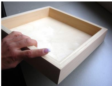
photo 4 - Panel Support This is the back of a panel support box as seen sitting on the table in photo 2. It is framed with 1/2" birch plywood glued with PVA white glue, not nailed. This supports the 1/4" maple face board.
