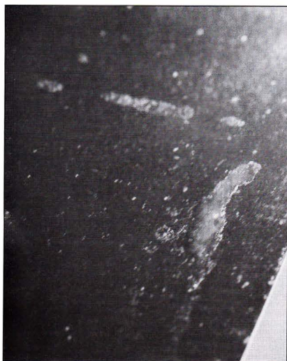
Photo 2: The press platen in this photo is just waiting to either transfer dirty adhesive or pattern indentations into an unsuspecting mounting project.
