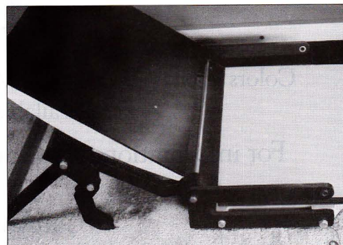
Photo 5: Once the bolts are removed, open the top of the press like a book to expose the coated platen for easy cleaning. Remember—never use anything abrasive on the surface to avoid scratching it.
