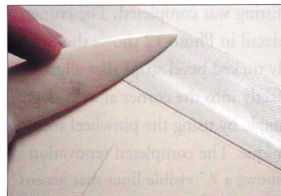
Photo 11: A strip of linen tape was used to book hinge the window mat unit along its longest side to the backing board. It was then burnished firmly to activate the adhesive.
