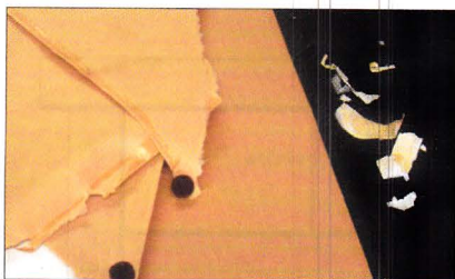
Photo 4: While the common worry about pressure-sensitive adhesives is that they will dry out, ooze, or soak in too aggressively, but these tapes and felt bumpers were still hanging on after 37 years.
