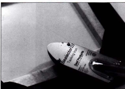
Photo 8: Mount the bark paper to the face of the created 8-ply blunt cut window opening, remove center, miter corners, and wrap to the back of the opening with a tacking iron.
