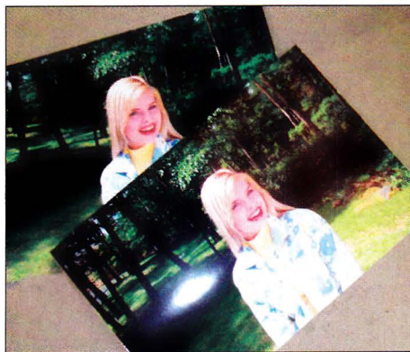
Photo 2: Fuji Autochrome—Fuji launched a new photo mini lab series called Printpix. It is the laser printing of digital photos. The images show the discoloration of the image when subjected to heat of dry mounting in a mechanical press. The image reverts back to its normal color within seconds of press removal, but the paper is slightly altered. So it seems heat sensitive, but with no lasting damage.
