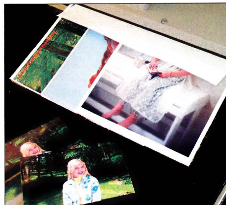
Photo 4: Heat Tolerances—I tested both the lower left Fuji Autochrome images and the Konica PhotoPapers using the mechanical press at 190°F for two minutes. There appeared to be no impact from the heat with the Konica samples.
