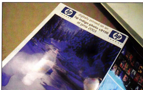
Photo 7: HP Indigo Heat Test—Though difficult to tell in this photo there was no color change when subject to temperatures of 190°F for two minutes. There was a slight visual alteration of the image glossed surface. It is no more disruptive than traditional orange peel though.
