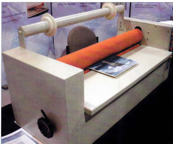
Photo 1: The Mini Mounter MM/225 is a newly released motorized, affordable cold roller machine with variable speed automatic or foot control, adjustable silicone rollers, forward and reverse gears, 25" wide, that adjusts to mounts up to 1" thickness from the Print Mount Company.
