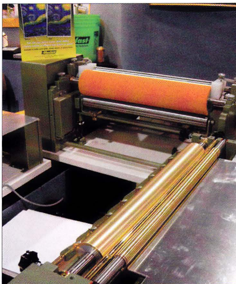
Photo 3: The Senator topside coater (center back) from Gluefast applies adhesive as well as being capable of coating the mounted art surface with acrylic sealers and textures. The Colonel electric gluer (right) evenly coats the artwork to be manually placed onto the substrate.
