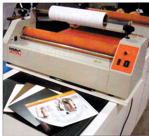
Photo 2: The JetMounter JM26 is one of a new series of 26", 43" or 53" cold mount laminators from Drytac with electric speed drive, silicone rollers, tension clutches (on JM43 and JM53), and all steel construction, which adjust to mount \frac{1}{2} " board substrate thickness. Also shown here is their new line of high tack pressure-sensitive boards.
