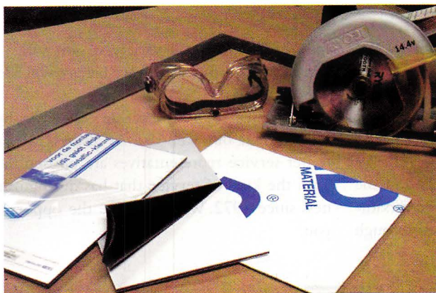
Photo 1: Dibond Cut to Size—Full sheets of the aluminum composite Dibond may be cut with a small rechargeable 5 1/2" skill saw. There are cover sheets on either side: one clear plastic, the other heavy lined.
