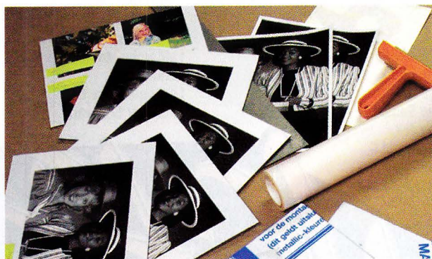
Photo 2: Mounting Tests—Test mountings included film RC photo, RC Cibachrome, Fuji Autochrome, Kodak Dye Sublimation, and Kodak black-and-white gloss images. (Upper right Crescent PerfectMount, center right Gudy 870.)
