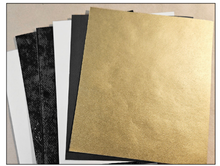
This shows the gloss of the premounted Beva that was hand ironed to each layer for a Surface Tiered (Precious Metal Gold and Black Canson) atop Pin-striped Tiered core of 4-ply cream ragmat (top and bottom) with 2 sheets of Black Canson between.
