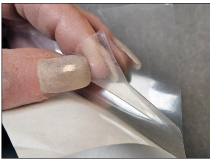
Beva film is sandwiched as opaque white 4mil silicone coated release paper, adhesive attached to a sheet of 1.5mil Mylar release film (Release paper + Adhesive + Mylar release film).
